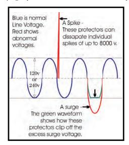
The ZAP-PRO protectors are *plug-in* devices that intercept most voltage problems **BE-FORE** they get a chance to do any damage to the circuit boards or components. The chart at left shows what AC waveforms look like on an oscilloscope, and also shows what some damaging transients might look like.
