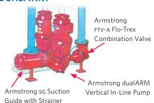
dualARM Vertical In-Line incorporates two pumps in a casing with single inlet and outlet connections. Enables standby or parallel operation with only one set of piping. Casing design and port valves allow one pump to be removed for service with the second pump still operating. When installed with a Suction Guide and Flo-Trex valve the dualARM represents the greatest Life Cycle Value in today's commercial HVAC market.
