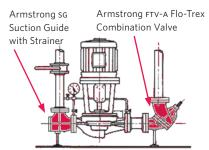
Vertical In-Line with Suction Guide and Flo-Trex valve eliminates cost and space of all the items listed under base mounted pump, plus the following:
