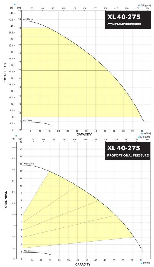
Note: The shaded area represents the operating range for the control mode. Each control mode will operate along a single control curve set by the max differential pressure set point.
