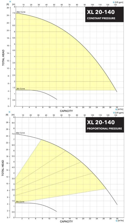
Note: The shaded area represents the operating range for the control mode. Each control mode will operate along a single control curve set by the max differential pressure set point.
