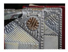
All damaged gaskets are then replaced and the plates are reinstalled in the same order they were removed. Our hydraulic rams are then used to recompress your heat exchanger back to factory specifications and dimensions.
