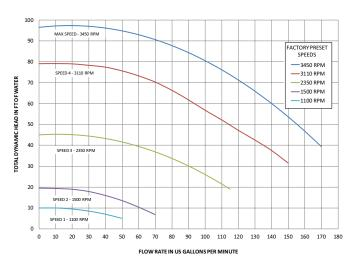
NOTE: The chart above demonstrates performance rates at factory preset speeds of 3450 RPM, 3110 RPM, 2350 RPM, I500 RPM and I100 RPM.
