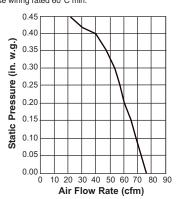
HVI-2100 CERTIFIED RATINGS comply with new testing technologies and procedures prescribed by the Home Ventilating Institute, for off-the-shelf products, as they are available to consumers. Product performance is rated at 0.1 in. static pressure, based on tests conducted in a state-of-the-art test laboratory. Sones are a measure of humanly-perceived loudness, based on laboratory measurements.
