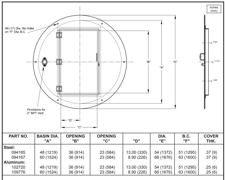
Basin covers have hinged access door, lifting handle, provisions for 2" NPT vent, stainless steel hinges and hardware. Covers have a load rating of 150 lbs/sq. ft. (732 kgs/sq. meter) minimum. Steel cover has Black Powder Coating.
