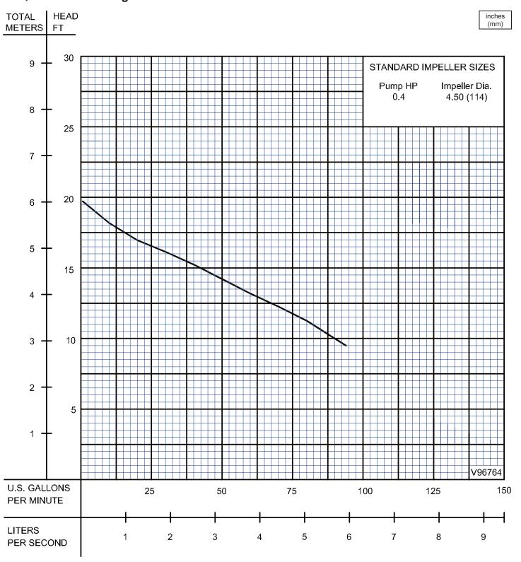
Testing is performed with water, specific gravity 1.0 @ 68° F @ (20°C), other fluids may vary performance
