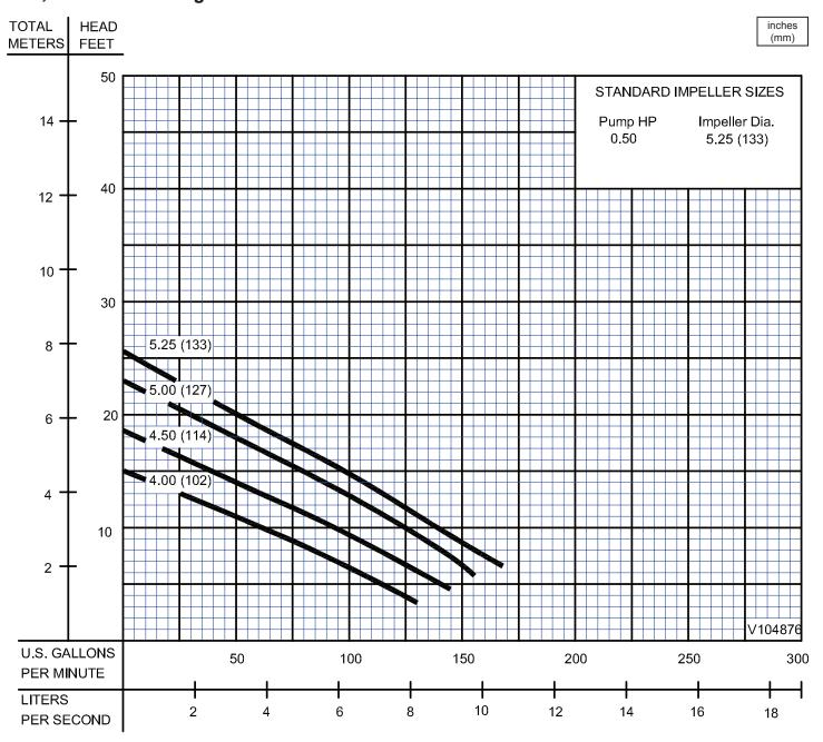
Testing is performed with water, specific gravity 1.0 @ 68° F @ (20°C), other fluids may vary performance
