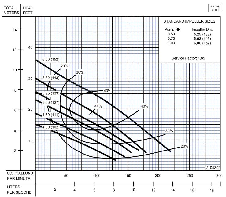
Testing is performed with water, specific gravity 1.0 @ 68° F @ (20°C), other fluids may vary performance
