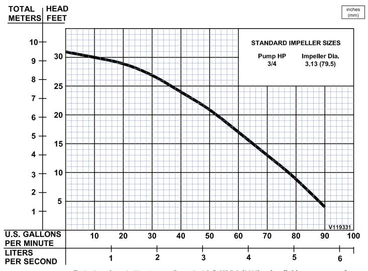
Testing is performed with water, specific gravity 1.0 @ 68° F @ (20°C), other fluids may vary perfor-
