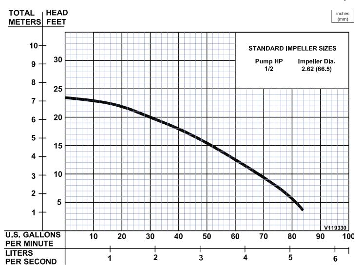
Testing is performed with water, specific gravity 1.0 @  $68^{\circ}$  F @ (20°C), other fluids may vary performance
