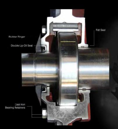
Ingress Protection – Contaminants and moisture can lead to early life failure of a motor Techtop has gone the extra mile in engineering a system of seals, gaskets and drains that protect our bearings and internal motor components from damage due to these foreign invaders. Wherever your Techtop moor finds itself it will be protected from the environment and ready for a long productive life.
