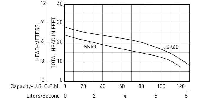
The curves reflect maximum performance characteristics without exceeding full load (Nameplate) horsepower. All pumps
