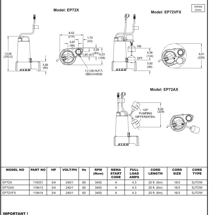
1.) PUMP MAY BE OPERATED "DRY" FOR EXTENDED PERIODS WITHOUT DAMAGE TO MOTOR AND/OR SEALS.
