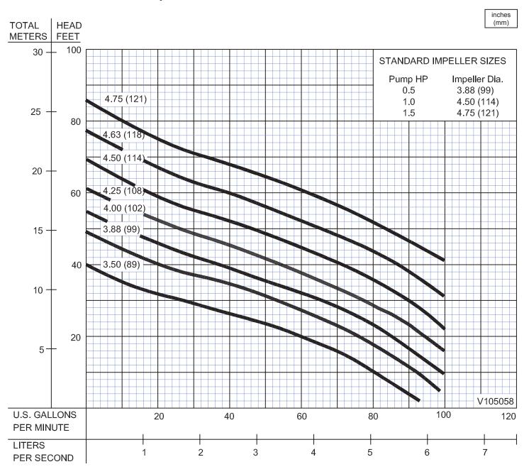
Testing is performed with water, specific gravity 1.0 @  $68^{\circ}$  F @ (20°C), other fluids may vary performance
