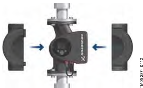
Fig. 57 Fitting the insulating shells to a MAGNA3 pump
