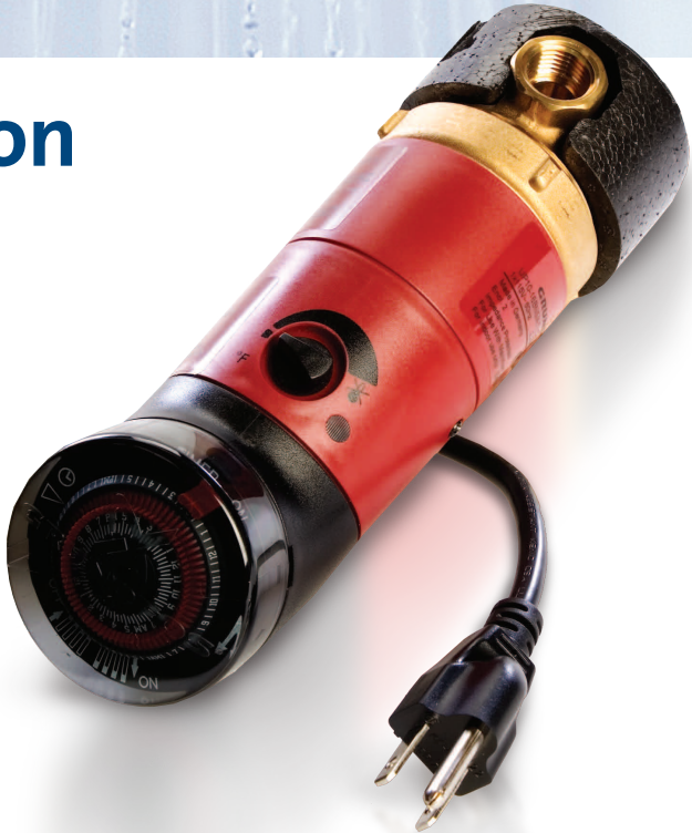
UP 10-16BU ATLC (Part# 96433899) Built-in timer, line-cord, and aquastat
