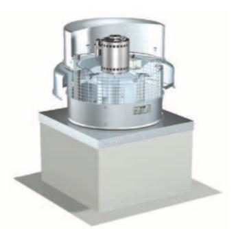
Spun aluminum downblast exhaust fans shall be direct drive-type. These fans are specifically designed for roof mounted applications exhausting relatively clean air. Performance capabilities range up to 4,300 cfm (7,306  $m^3/hr$ ) and 1 in. wg (249 Pa) of static pressure. The maximum continuous operating temperature shall be 180°F (82°C). Model G fans are available in sixteen sizes with nominal wheel diameters ranging from 7 to 18 inches (178 to 457 mm) (060-180 unit sizes).
